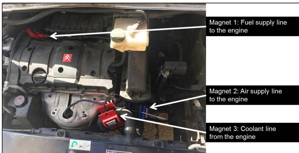
Figure 2: Magnets fitted in the car
